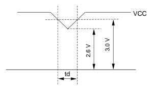
\*2) VCC = +3.3 V , f\_H=31.7 kHz, fv=60 Hz, fclk=30.4 MHz
