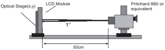
FIG. 1 Optical Characteristic Measurement Equipment and Method
