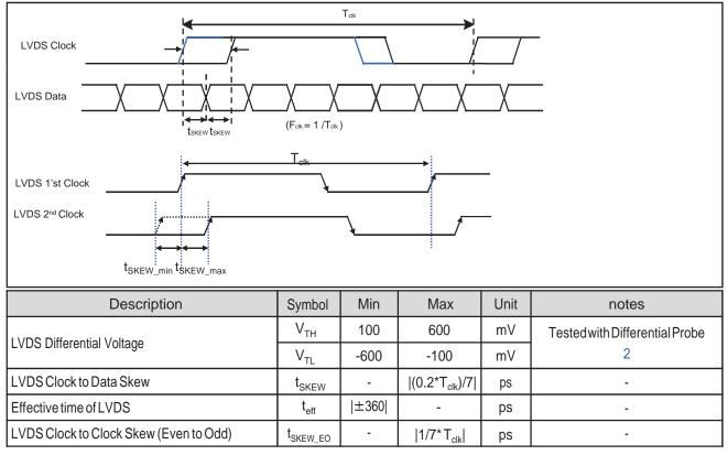
notes 1. All Input levels of LVDS signals are based on the EIA 644 Standard.
