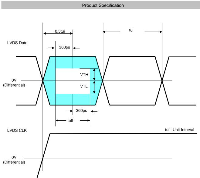
\* This accumulated waveform is tested with differential probe
