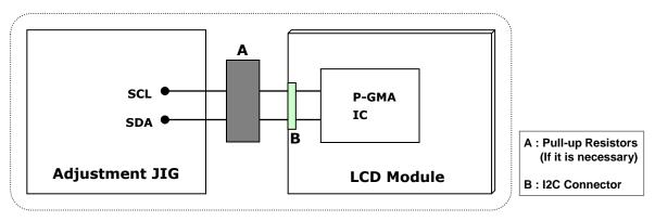
FIG. 8 VCOM Adjustment Pattern & Block Diagram
